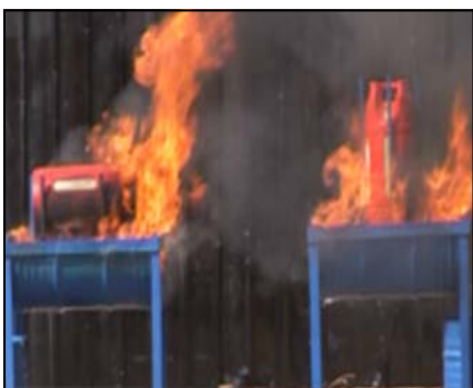
LPG cylinder 85% filled with propane and subjected to intensive fire.
