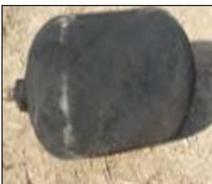
Advantex® 158B roving over wrap shows no external damages after passing the test
